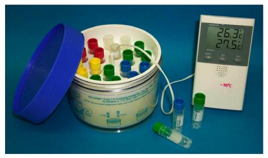
Figure 16. Slow freezing using Nalgene<sup>™</sup> cryo 1°C Freezing Container with temperature probe.
