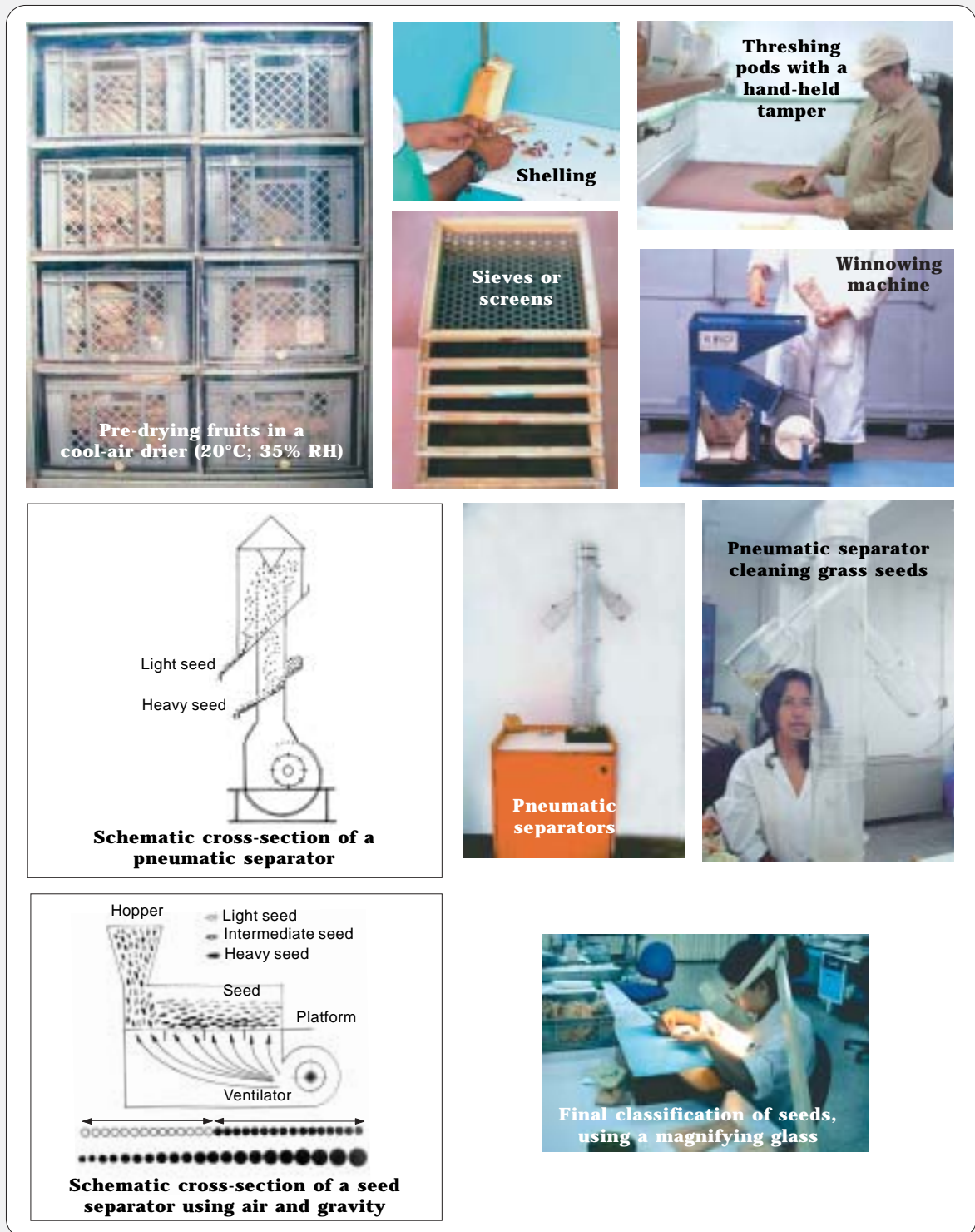
Figure 1. Conditioning seeds. Procedures and equipment used (photographs by B Pineda, GRU, CIAT; diagrams from CIAT 1989).
