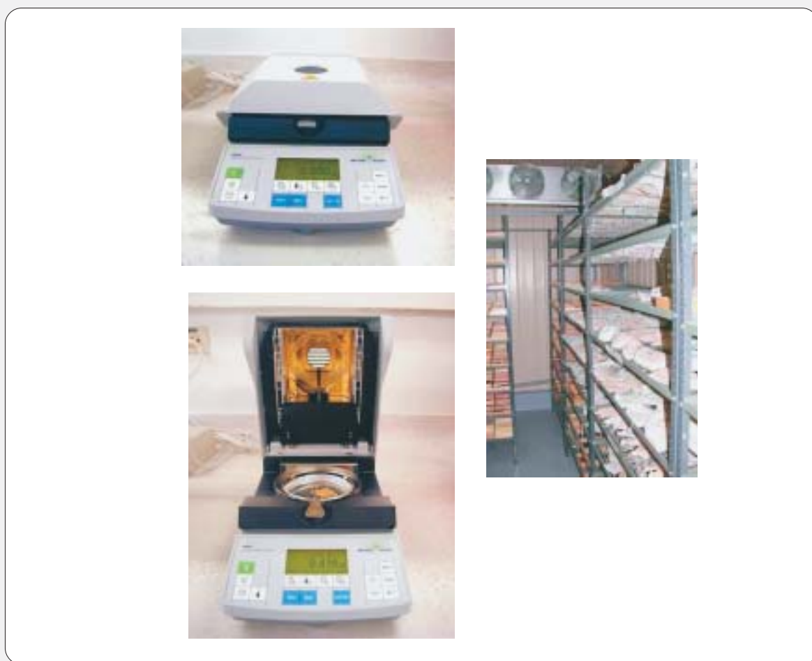
Figure 2. Drying seeds. Left, balances to determine seed moisture content and, right, cool-air drying room (20°C; 22% RH) (photographs by B Pineda, GRU, CIAT).
